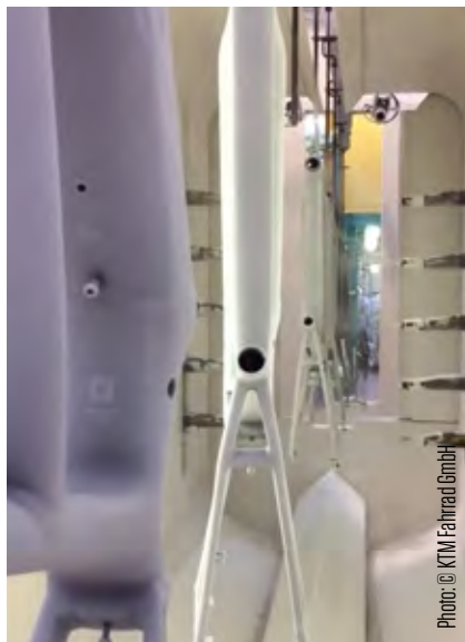
THE PRIMER AND FINISH ARE APPLIED TO THE BICYCLE FRAMES IN THE FULLY AUTOMATED POWDER COATING LINE.
